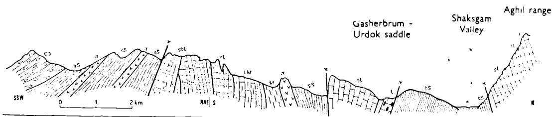
Fig. 24 - Geologic section along the crest dividing the Urdok from the Sgan and the Nakpo (Gasherbrum) glaciers.
